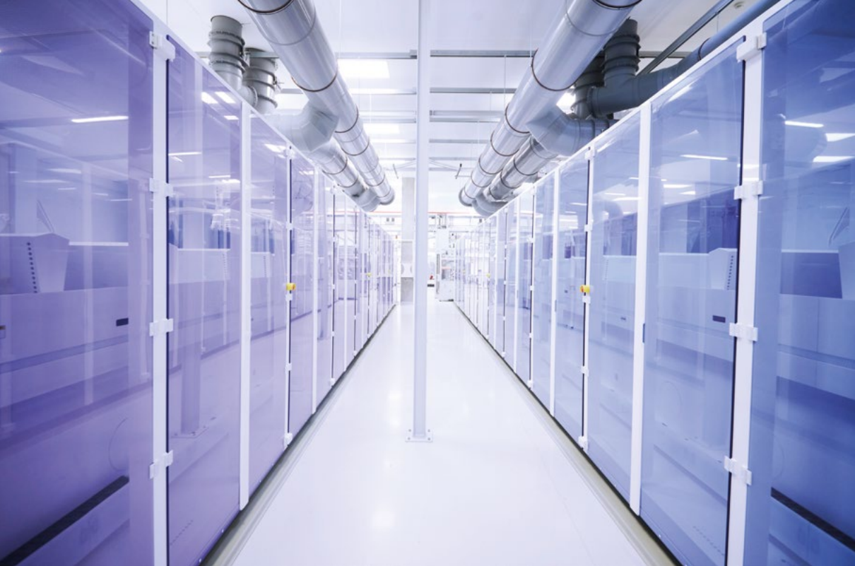
Fig. 34 In wet chemistry, the wafer is prepared for processing ©Meyer Burger
