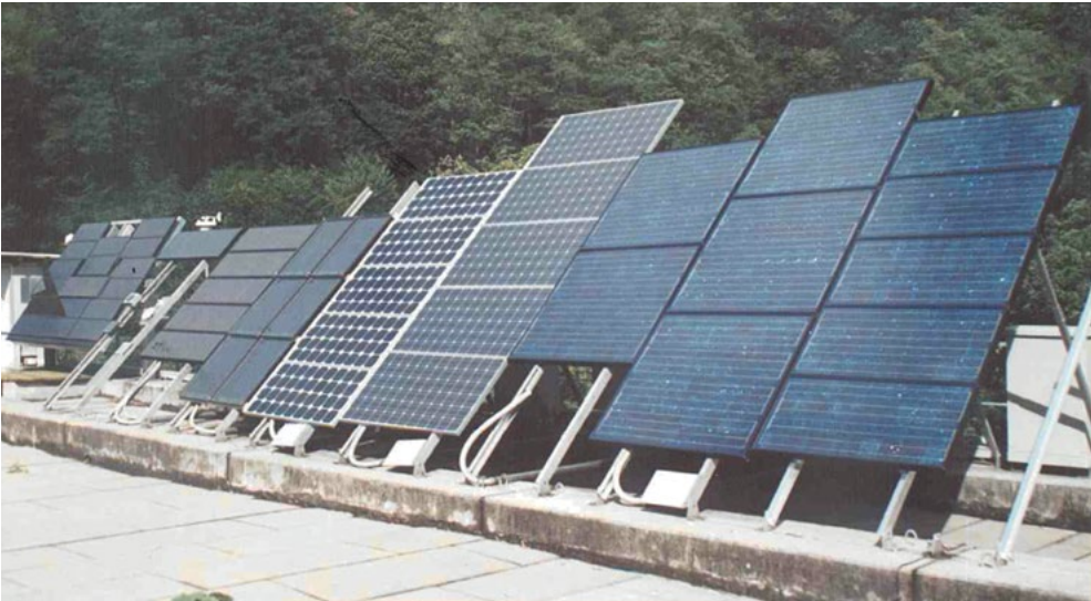
Fig. 07 Outdoor test stand (1995) - TISO research group @SUPSI
