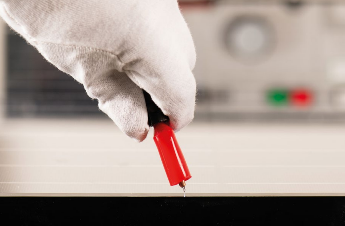
Fig. 22 SUPSI PVLab - Insulation test ©SUPSI Fig. 23
