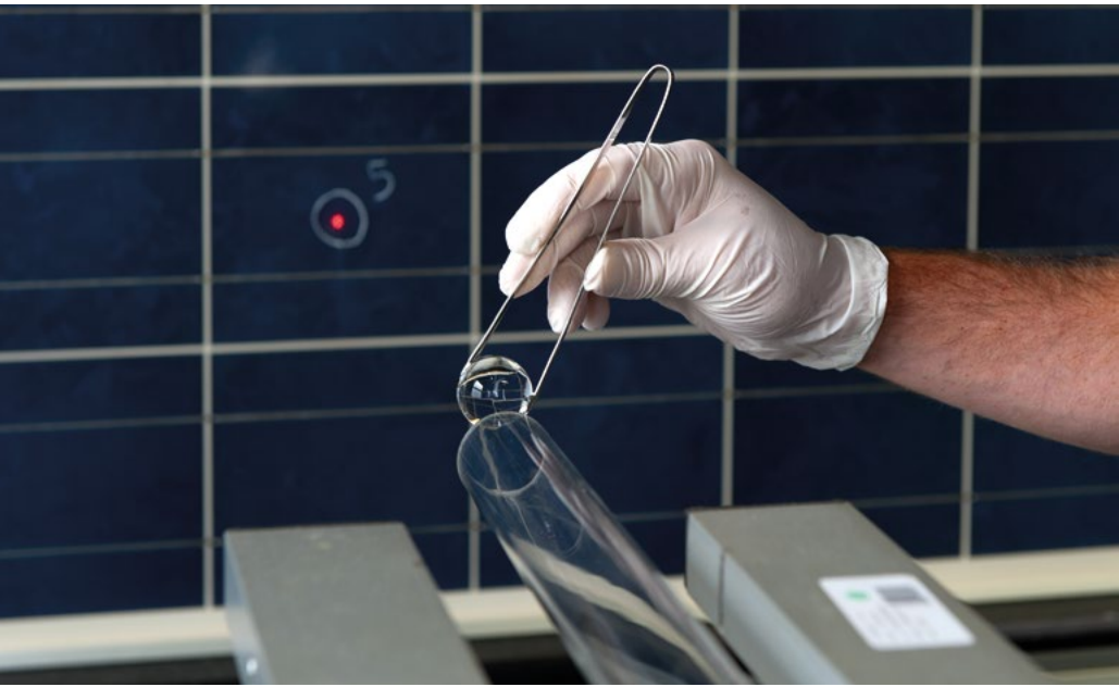
Fig. 27 SUPSI PVLab - Hail test: loading of the hailstone and target placement ©SUPSI Fig. 28 BELOW. SUPSI PVLab - Module breakage test ©SUPSI
