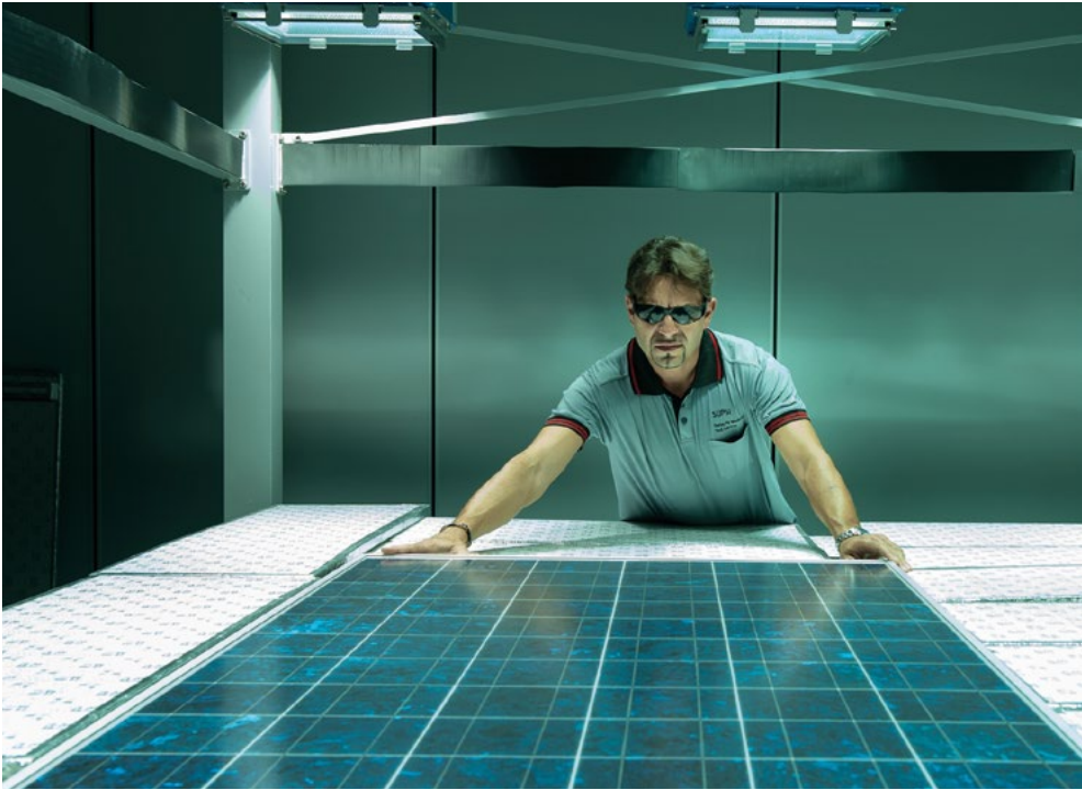
Fig. 24 SUPSI PVLab - Stabilization of a PV module under the light soak bench ©SUPSI Fig. 25 RIGHT. SUPSI PVLab - Accelerated testing in the UV chamber ©SUPSI
