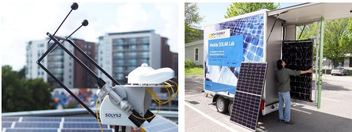
Figure 112: (left) Solar irradiance monitoring, including diffuse horizontal irradiance (DHI), direct normal irradiance (DNI), mounted south of tracker. (right) Modules are characterized by triple A+ Mobile Solar Simulator.
