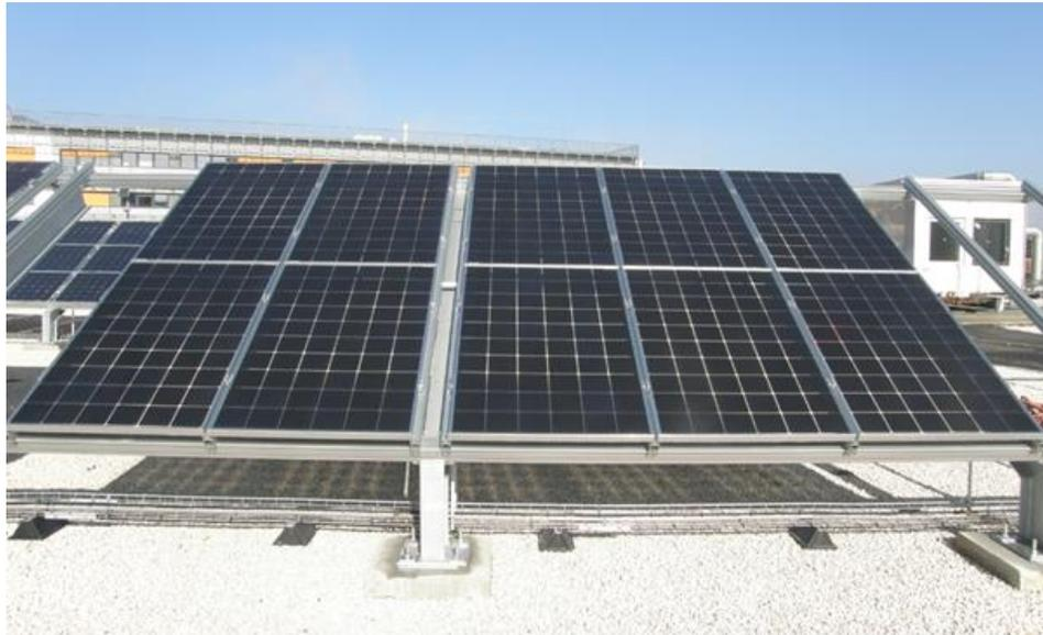
Figure 70: Front view of PV bifacial modules under test at INES site.
