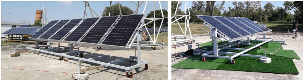
**Figure 107: Bifacial PV system under test; South-facing PV module on light grey concrete tilted 30°(left); South-facing PV modules on synthetic green grass tilted 30° (right).**
