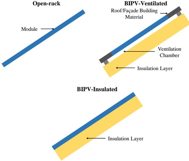
Fig. 1. Summary of installation configurations on the BIPV test stands.
