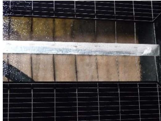
Viganello: HJT glass/glass module showing darkening of the contacts and delamination of fingers at the module border
