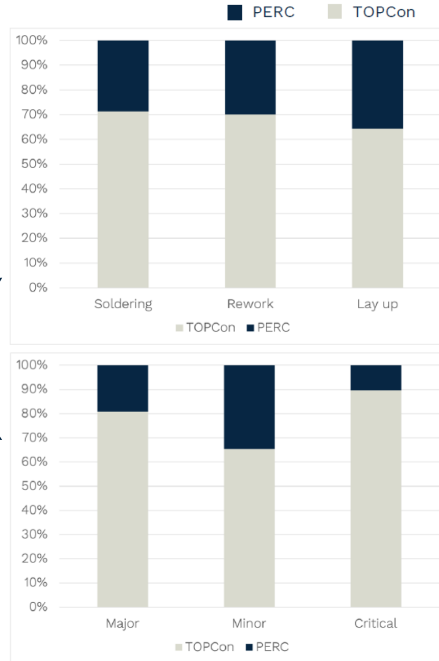
Defect ratios by cells type
